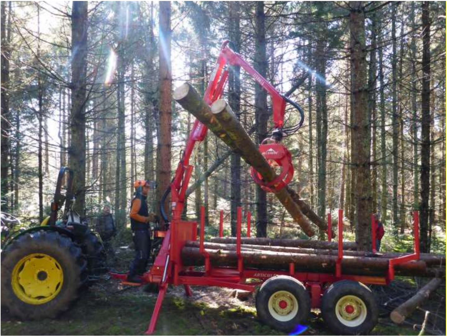
Loading small-diameter spruce logs during a plantation thinning demonstration at NorthWoods. Small forwarding equipment is ideal for working in dense stands such as this, where the articulated steering axle and ability to maneuver logs between trees minimizes damage to growing stock.
