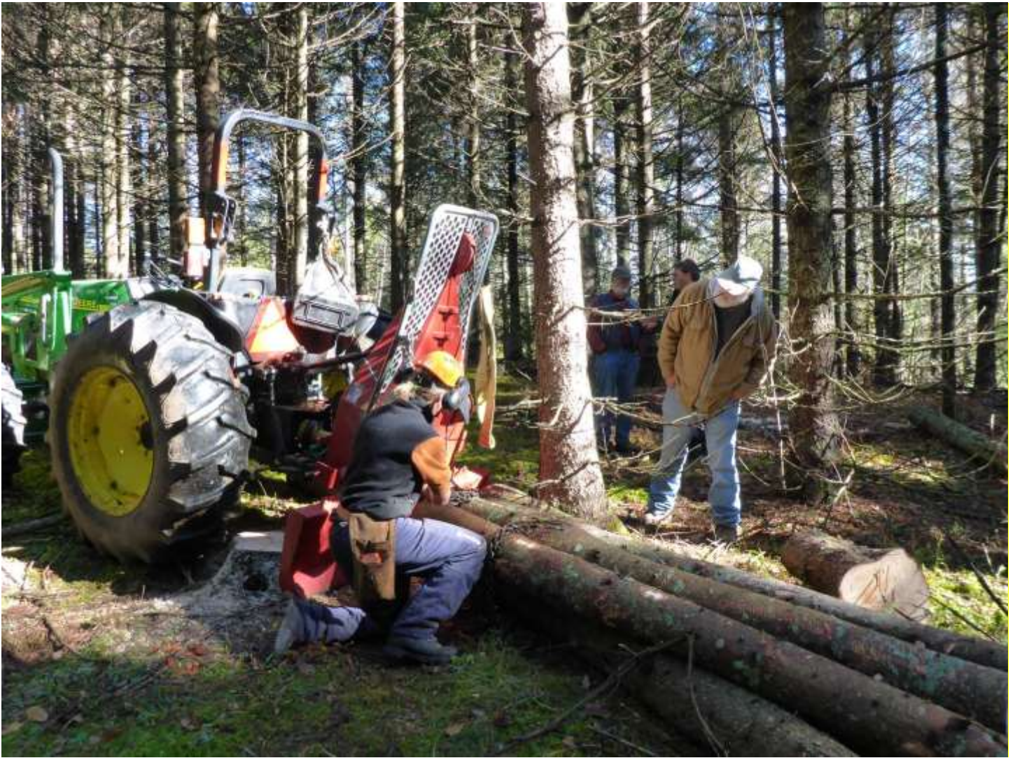
Winching logs to a trail during a plantation thinning demonstration at NorthWoods while a program participant watches. By winching logs 50-100 feet to a trail where they'll be collected with the forwarder (rather than driving to each log), area of soil compaction and damage to understory plants is greatly reduced.
